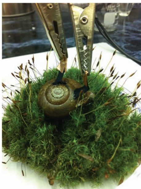
Figure 2. Photograph of a snail with implanted biocatalytic electrodes connected with crocodile clips to the external circuitry (close view).
